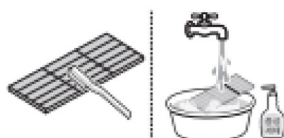
Figure 22: Cleaning the Filter and Heat Exchanger Element.
