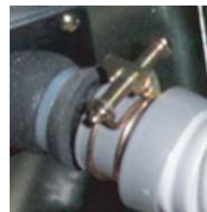
Figure 72: Flexible Drain Hose Connection.
