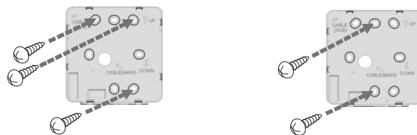
Four-Socket Handy Box Installation Two-Socket Handy Box Installation
