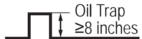
Figure 57: Close Up of An Inverted Oil Trap.
