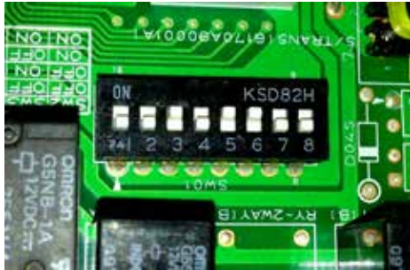
Figure 56: Hydro Kit Medium Temperature DIP Switch Block
