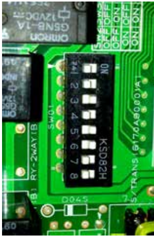
Figure 57: Hydro Kit High Temperature DIP Switch Block
