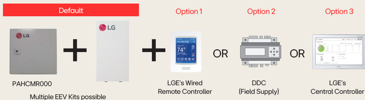
Figure 8 - Communication Kit Combination
