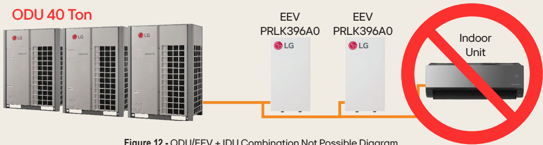
Figure 12 - ODU/EEV + IDU Combination Not Possible Diagram
